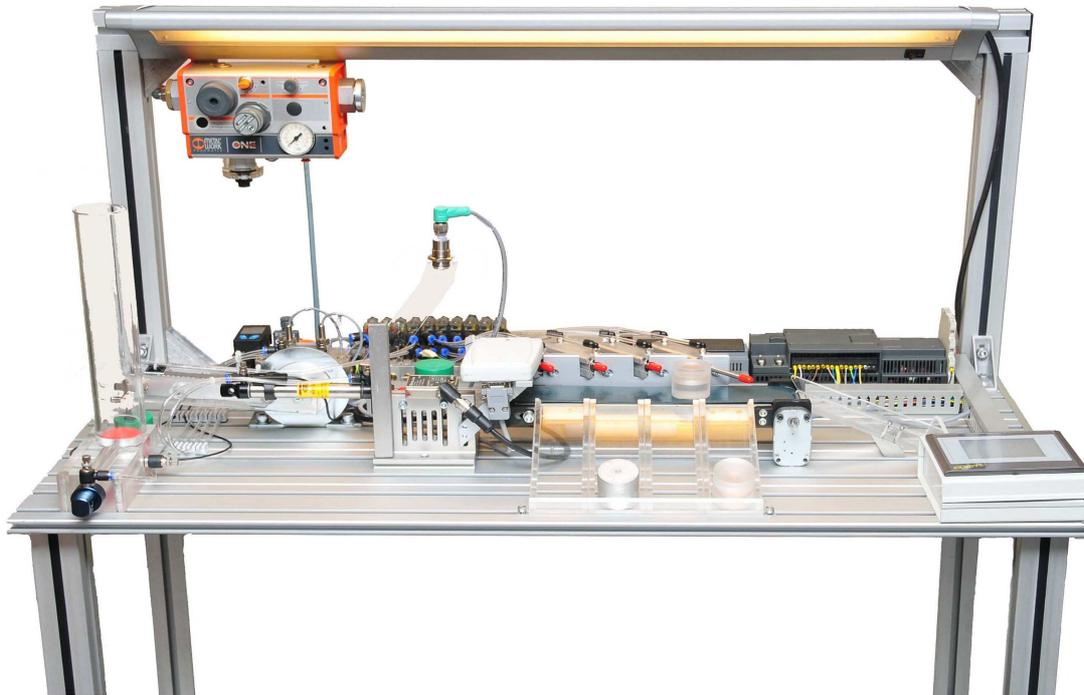
The objective of Ferma Mechatronics Training Set is to show students how to deal with various types of sensors and how to set an algorithm with a PLC.
