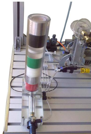
RF tag reader can read 4 samples and separate them according to the predefined sections.
