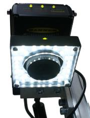
The use of cameras instead of sensors is the new technology in object recognition. Objects are scanned through an intelligent camera. The camera is programmable and does the image processing by itself. Here in this training set, the camera recognises (“reads”) the letters at the first row and sends the data to the PLC in ASCII format. The PLC takes the positions of each letter in memory. The user types on the touchscreen what to “write” on the second row.
